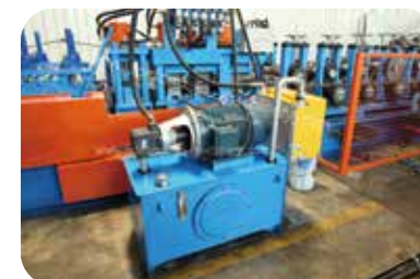
⑩ 液压站 Hydraulic Station
