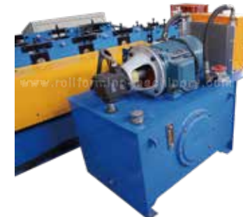
⑩ 液压站 Hydraulic Station
