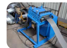
放料伺服一体机 Discharging servo all-in-one machine
