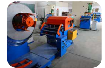
放料伺服一体机 Discharging servo all-in-one machine
