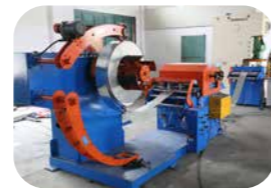
放料伺服一体机 Discharging servo all-in-one machine
